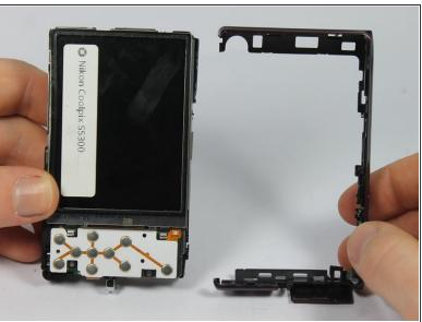
Carefully remove the top button casing by pulling it away from main camera.
