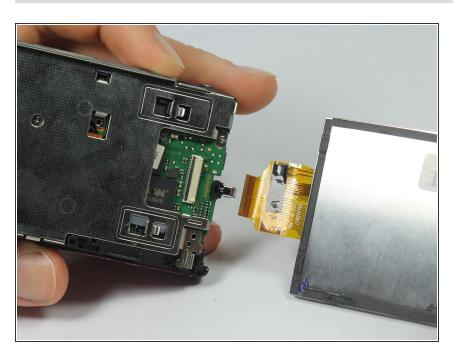
Once the ribbon cable is disconnected, remove the LCD screen.
