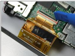
To disconnect the ribbon cable, use the tip of a plastic opening tool or your fingernail to flip up the small retaining flap. Then, you can safely pull the ribbon cable out.
