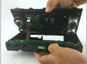
• Use a metal spudger to pry the device apart. You must use a metal spudger because of the great force necessary to pry it apart.
