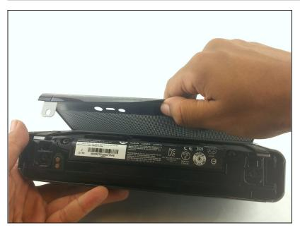
Flip the rear panel back to allow access to the SoundLink's battery.
