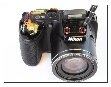
Remove the two 1.5x2.5mm screws below the flash unit using a PH000 screw head.
