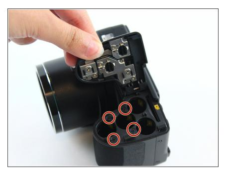
Remove the four 1.5x2.5mm screws in the battery housing using a PH000 screw head.
