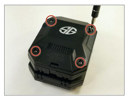
Unscrew Top Cover with a 3mm Triangle driver bit from the Driver Kit.
