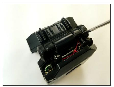
• Release pilot studs near the hinge with Metal Spudger.
