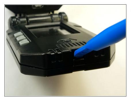
• Use Opening Tool to release barbed latch on top cover.
