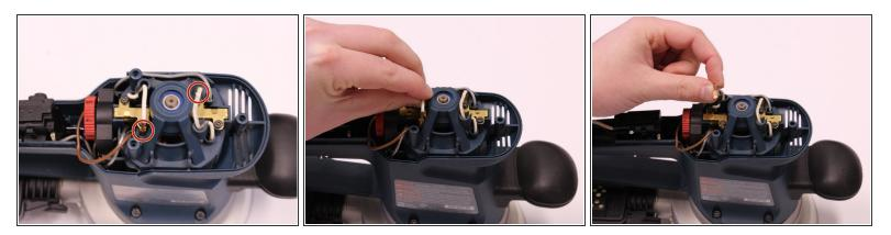
• Remove the two white wires connected to each motor brush by pulling on the spade terminals.
