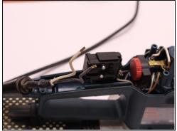
Using the <u>2.5 mm Flathead</u> Screwdriver, loosen the two screws securing the white and black wires to the On/Off Switch.
