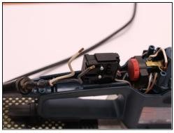
Using the <u>2.5 mm Flathead</u> Screwdriver, loosen the two screws securing the white and black wires to the On/Off Switch.
