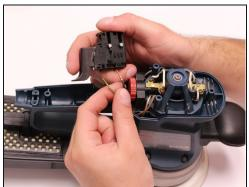
• Remove the gray and purple wires by pulling on the wire terminals.
