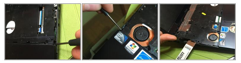
• Pry in the 2 points. Using a flat tool release the trackpad block along the perimeter
