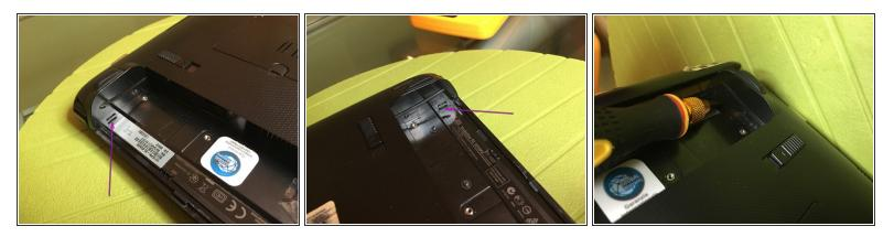
use a screwdriver to press in the 2 slots to unlock the keyboard hooks
