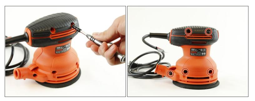
Use the TR20 Torx Security bit driver to unscrew the five 18.75mm Phillips screws from the warning label side of the chassis.
