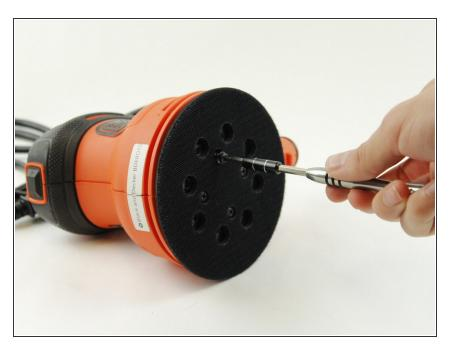
Select the JIS - J1 bit or the most appropriate bit to match the screws for your model.
