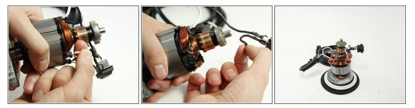
• Gently pull on all cables connected to the motor to remove.
