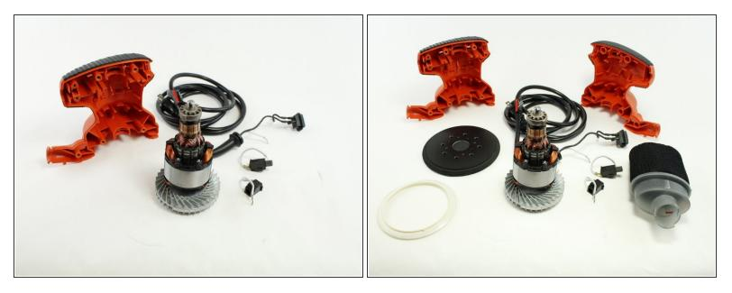
• Once all cables are disconnected, you can proceed to replace the motor.
