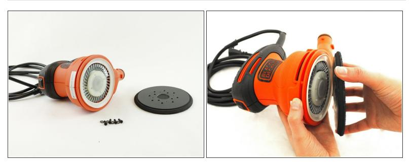
Once all screws and washers have been removed, hold the hook and loop system and separate it from the device.
