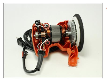
Identify the white cables connected to the holder brush and spring.
