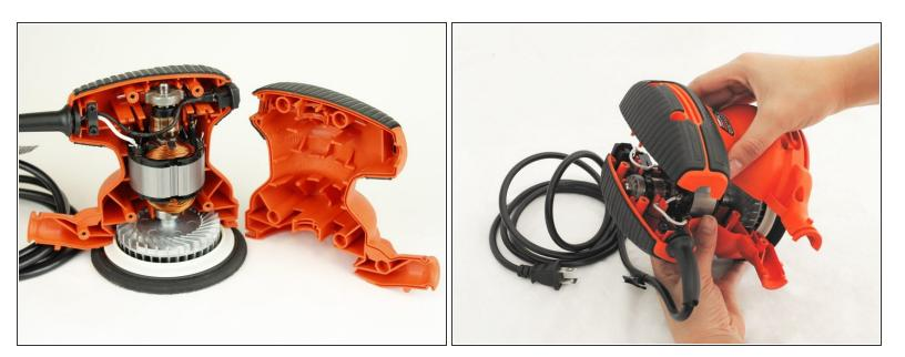
• Hold the chassis and separate it from the device.
