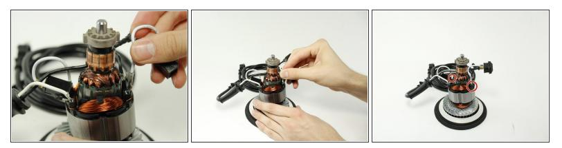
Remove the wire connected to the brush holder from the motor by pulling gently.
