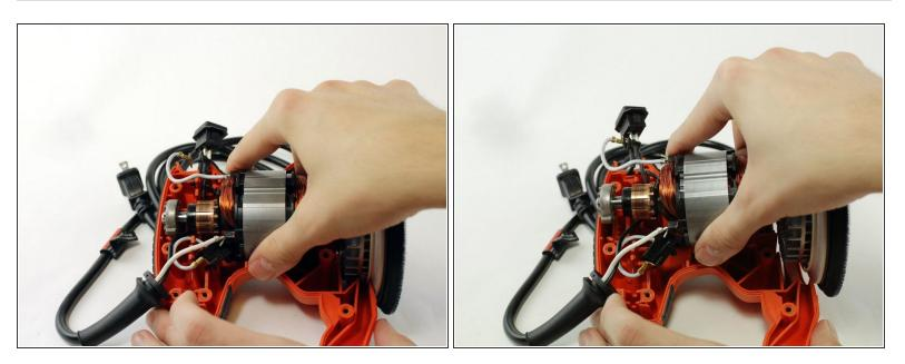
• Hold the motor and gently pull to remove from chassis.
