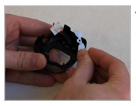
Remove the metal plate that holds the microphone.
