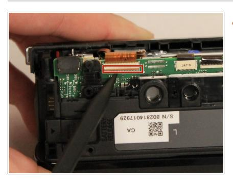
Using the spudger, pull the tab shown to start removing the ribbon cable.
