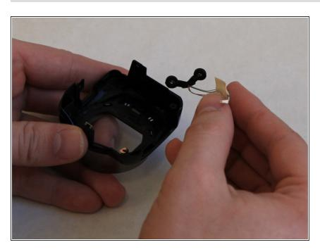
Remove the defective microphone out of the lens cap.
