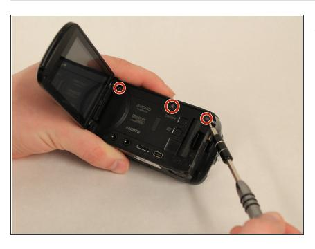
Near the LCD screen, remove the three 7mm Philips #000 screws in the picture shown.
