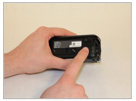
• On the bottom of the battery hold the battery release switch.
