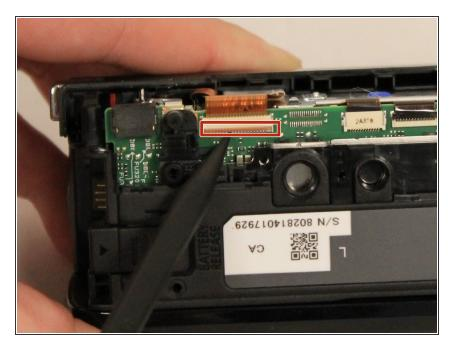
Using the spudger, pull the tab shown to start removing the ribbon cable.
