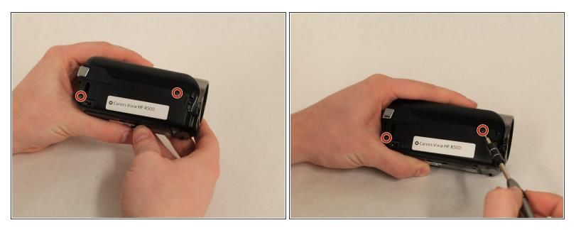
• Remove the two 8mm Philips #000 screws on the side where the grip belt was located on.
