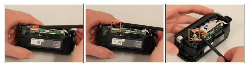
Using the Spudger, carefully remove the two ribbon cables that are connected to the top of the device.
