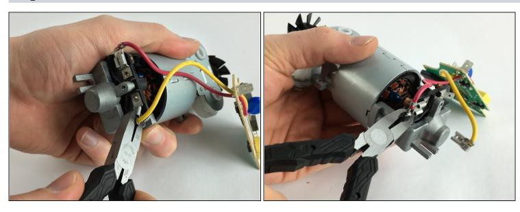
• Firmly grip the motor in your hand. Using pliers, pull the connectors off the motors.
