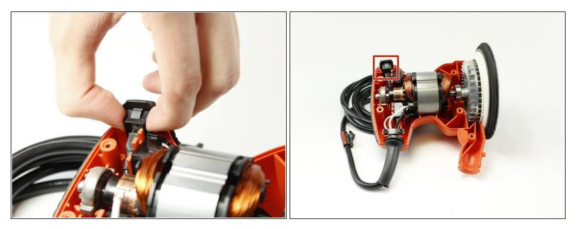
• Hold the power button and pull it out of the chassis.
