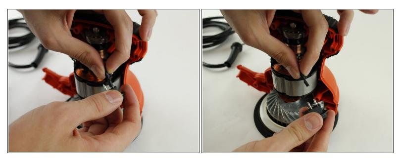
• Detach the black wire connected to the power button from the motor. To do this, gently pull the cable while holding the power button.
