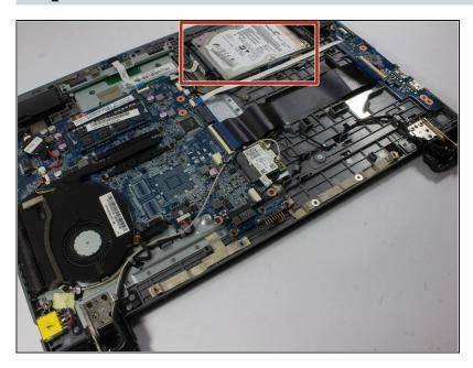
Locate the hard drive assembly on the top right hand corner of the Flex 15 based on the orientation of the device in the picture.
