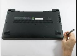
• Working your way around the outer edges of the Flex 15, remove the 8 (30 mm) outer screws.
