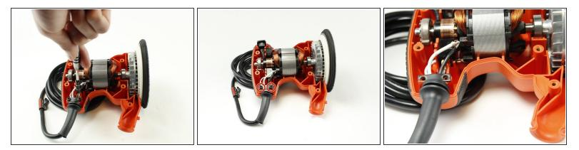
Use the bit driver with the JIS - J1 bit to remove the two 12.5 mm phillips screws holding the cord clamp to the chassis.
