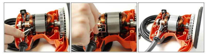
• Gently pull the white cable that connects the power cord to the motor to detach it.
