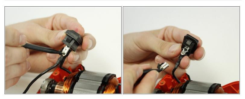
• Push the security pin with the plastic spudger and simultaneously, pull gently on the cable to separate it from the button.
