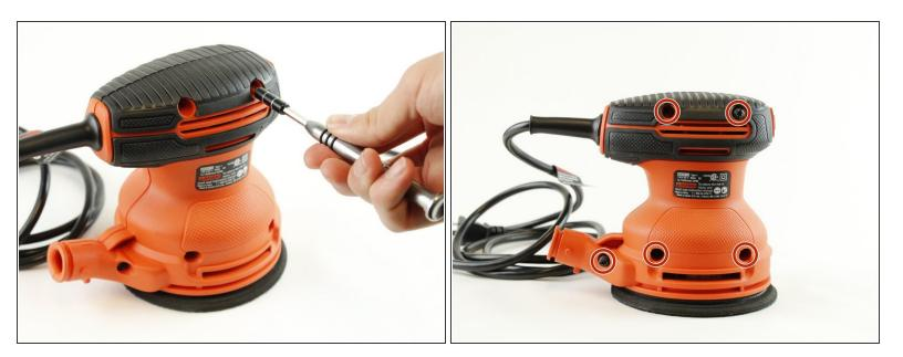
Use the TR20 Torx Security bit driver to unscrew the five 18.75mm Phillips screws from the warning label side of the chassis.
