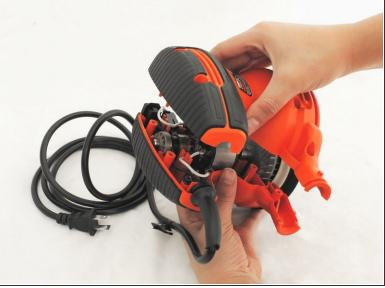
Hold the chassis and separate it from the device.
