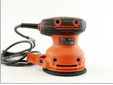
Use the TR20 Torx Security bit driver to unscrew the five 18.75mm Phillips screws from the warning label side of the chassis.
