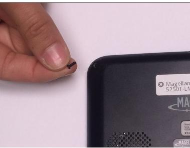
Remove all four 5 mm screws from the back of the device using a Phillips Head screwdriver size 000.
