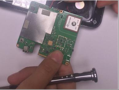
Remove the motherboard from the device by unscrewing all three 4 mm screws that are connecting it to the casing with a Phillips Head screwdriver size 000.
