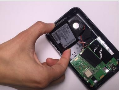
Pry off the original battery using a spudger to break the adhesive that connects the battery to the back casing.
