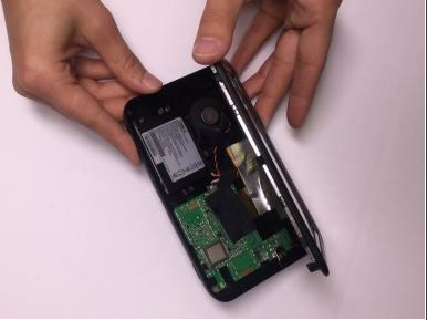
Open the casing of the device using a plastic opening tool.
