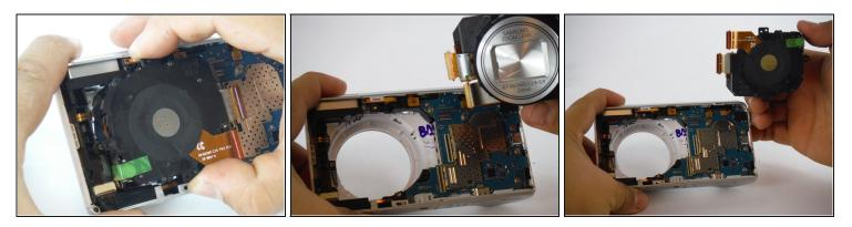
• Now that the screws and ribbon cables have been removed, gently pull the lens assembly up from the the camera and remove it.
