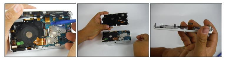
• With the screen separated from the main chassis, use the plastic opening tool to gently pry the edge of the ribbon cable connector from the motherboard.
