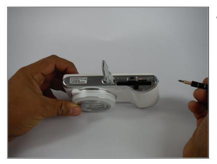
• Use the screwdriver to remove screws listed in step 2. There are a total of six 4mm screws.
