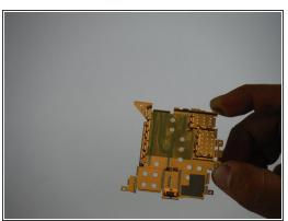
• Underneath the motherboard, there is a thin metal plate. This plate should lift up easily, as there are no screws keeping it in place.
