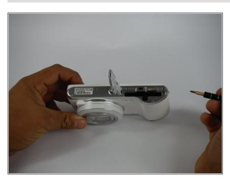
Use the screwdriver to remove screws listed in step 2. There are a total of six 4mm screws.
