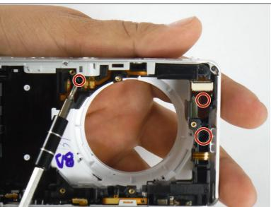
Now, all that's left is the frame and black interior frame. To get to the flash assembly, the black frame must be entirely removed.
