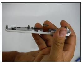
With the screen separated from the main chassis, use the plastic opening tool to gently pry the edge of the ribbon cable connector from the motherboard.
