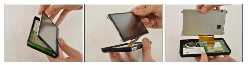
• Gently lift up the display screen using your fingers to make sure the only thing connecting it to the body is the ribbon cable.
