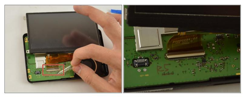
• Remove the piece of tape that is covering the connecting point of the motherboard and display.
