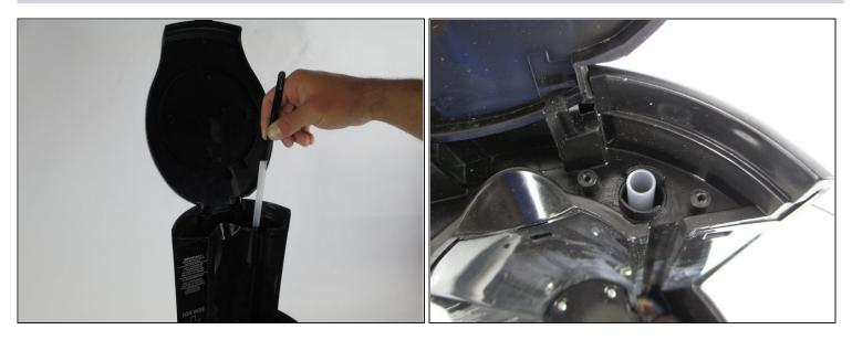
• Using <u>tweezers</u>, grab the tube that is exposed after you pulled the piece off in step 1 and pull it up and out of the Brew Station.
