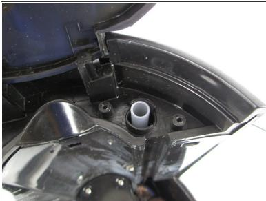
• Using tweezers, grab the tube that is exposed after you pulled the piece off in step 1 and pull it up and out of the Brew Station.
