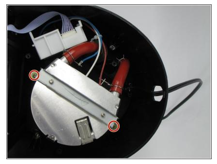
Using the Philips 2 Screwdriver, unscrew the two 8-mm screws labeled in a red outline. This will release the bracket that is holding down the large piece in the middle.
