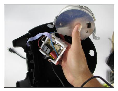
Once the screw is out, gently lift the white circuit board out of the base.
