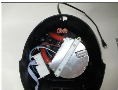
Using the Philips 2 Screwdriver, unscrew the two 8-mm screws labeled in a red outline.
