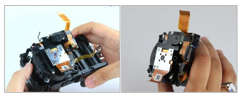
• Gently push the lens barrel up and out of the case.
