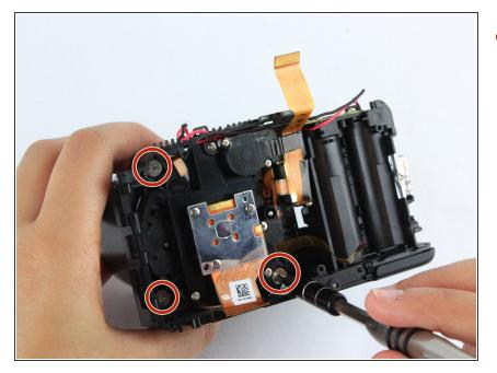
Remove the three 2.90x1.75mm screws using a PH000 screw head.
