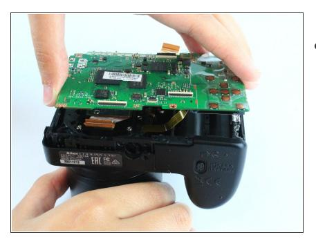
Remove the motherboard by lifting it directly up.
