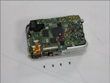
• Locate four black 3.0 mm screws on the motherboard and remove them using a Phillips screwdriver with a #0 bit.
