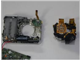
Grasp the lens assembly and carefully lift it out of the camera.
