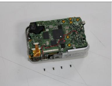
• Locate four black 3.0 mm screws on the motherboard and remove them using a Phillips screwdriver with a #0 bit.
