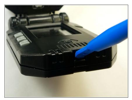
Use Opening Tool to release barbed latch on top cover.
