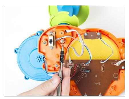
Use Phillips #2 screwdriver to loosen and remove the single 16 mm screw.
