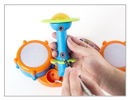
Loosen and remove the two 14 mm screws using a Phillips #2 screwdriver.
