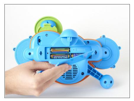
Using your fingers, pry open and remove the back battery panel.
