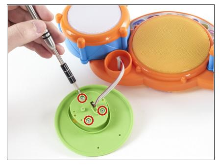
Using a Phillips #00 screwdriver, loosen and remove the three 12 mm screws located on the bottom of the green cymbal.
