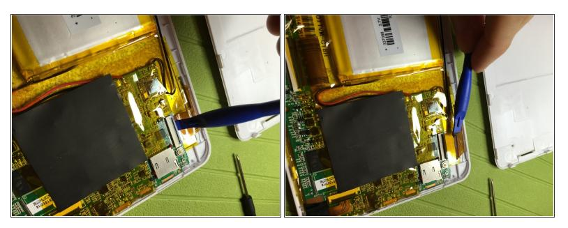
lift the lock on the touch screen connector
