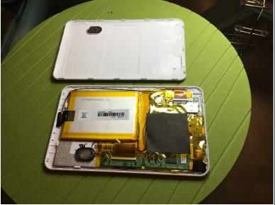
remove back cover with the help of a thin tool
