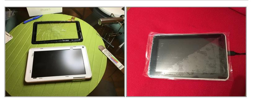
completely remove the broken glass and replace it with the new one
