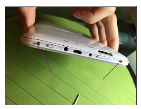
Remove the 2 screws on the bottom of the device, arrows
