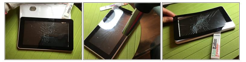
with the help of a heat source and a thin tool remove touch screen
