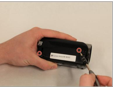
Remove the two 8mm Philips #000 screws on the side where the grip belt was located on.
