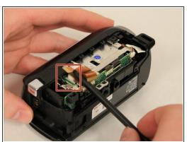
Using the Spudger, carefully remove the two ribbon cables that are connected to the top of the device.
