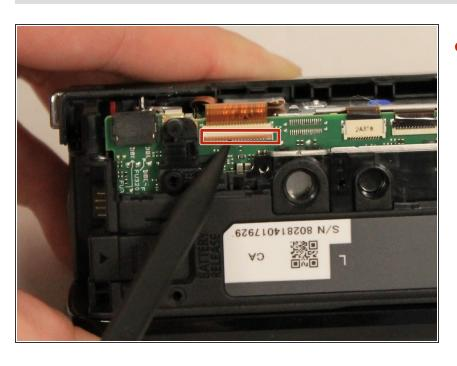
Using the spudger, pull the tab shown to start removing the ribbon cable.
