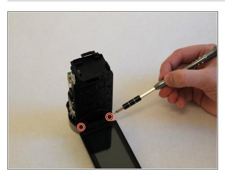
Remove the two 5mm Phillips #000 screws near the LCD screen.
