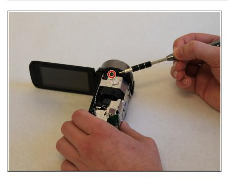
Remove the single 5mm Phillips #000 screw located on the top of the camera near the lens cover.
