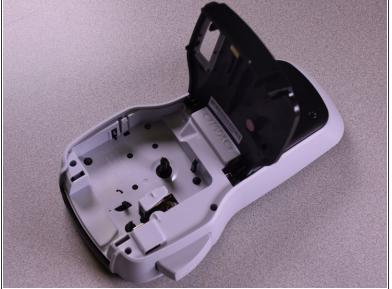
Open the label cartridge compartment and remove any current label cartridge to reveal your label cutting blade.
