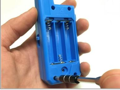
• Using your Phillips head screwdriver, unscrew all four 4mm screws from each corner.
