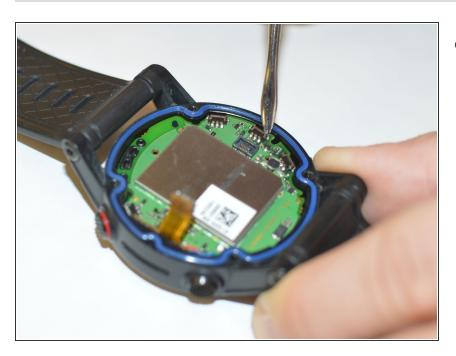
Use the spudger to pry the motherboard out of the housing.
