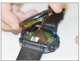
Use a Torx T9 screwdriver to remove these four .8mm screws and seperate the housing.
