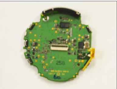
• Lastly use your spudger tool to pry the data ribbon open from the motherboard. Once the ribbon is removed the board will be free and you can replace the board.
