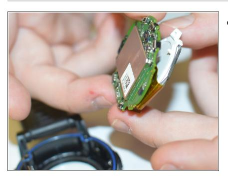
Once removed simply separate the digitizer from the main board.
