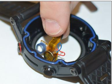
Use a spudger tool to pry the soundboard out of its housing.
