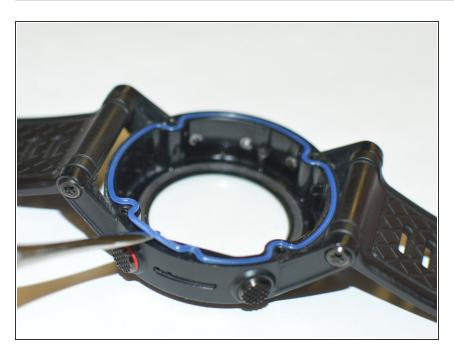
Remove the gasket seal from the housing.
