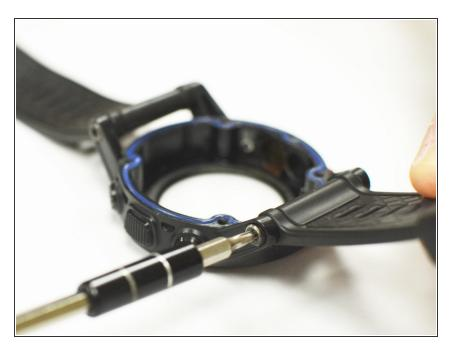
Use a Torx T9 screwdriver to remove the four .8mm screws. Once the screws are removed the watch straps should fall out of the housing.
