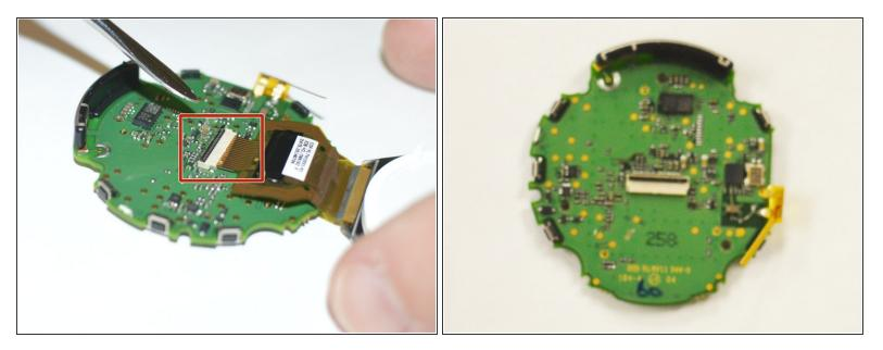
Lastly use your spudger tool to pry the data ribbon open from the motherboard. Once the ribbon is removed the board will be free and you can replace the board.
