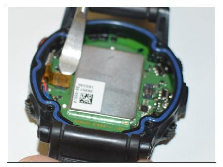
• Use a spudger to pry open the power ribbon from the main board.
