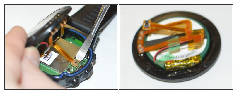
• Use a spudger tool to disengage the power ribbon from the main board. Once the ribbon is disconnected you can separate the bottom piece of the housing that holds the battery.
