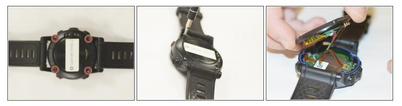
Use a Torx T9 screwdriver to remove these four .8mm screws and seperate the housing.
