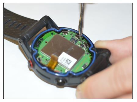
• Use the spudger to pry the motherboard out of the housing.
