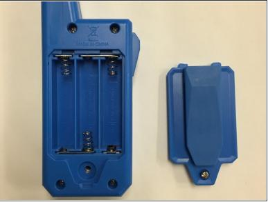
Remove the battery cover. Replace the old batteries with the new ones.
