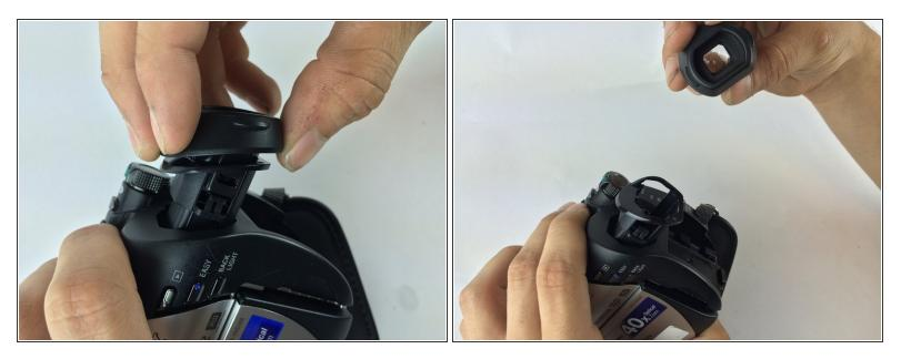
Once loosened gently pull and remove lens housing. The lens should now be free to inspect and replace.
