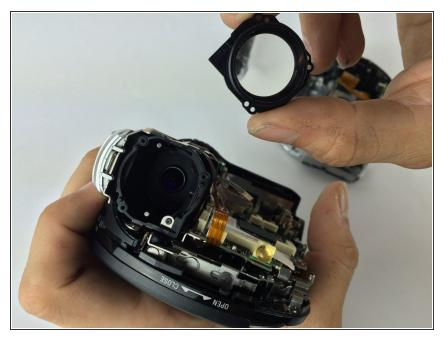
Remove front lens and inspect for "dirt," smudges. or scratches. Use discretion, if lens appears too damaged, replace part.
