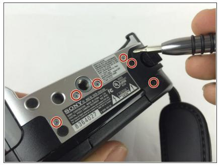
Remove all the 4.3mm screws on the bottom using a J000 Phillips screwdriver. There should be seven screws (4 silver, 2 black).
