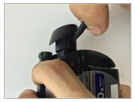
• With the pointed end of a plastic spudger, press latch located on the side of rear lens housing.
