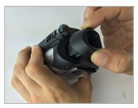
• Gently pull lens housing to expose housing channel.
