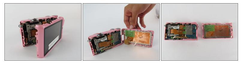
• Separate the LCD half compartment of the camera from the main body.
