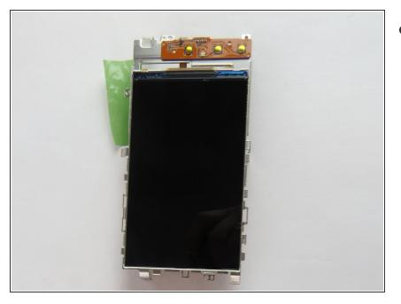
• The LCD screen is now separated form the main frame.
