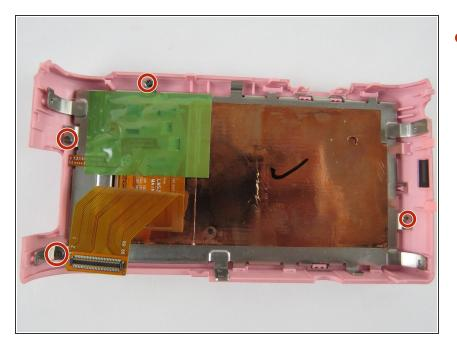
Remove the four 1mm screws with the Y0 screwdriver.
