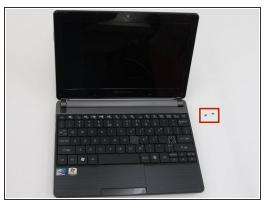
• Unscrew the two 5.0mm screws underneath the screen covers on the left and right side and remove them from the laptop. For this step and the following steps, use a Phillips #0 head screwdriver.
