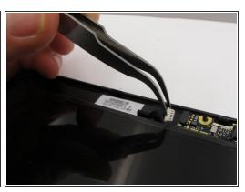
Unplug the webcam connection from the top of the laptop screen backing.
