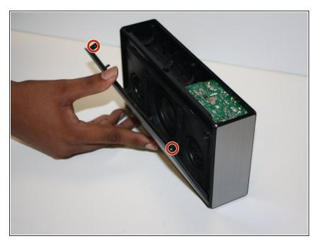
Remove the speaker grill by pushing on the two tabs in the corners.
