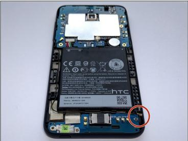
Using <u>Tweezers</u>, disconnect antenna wire.
