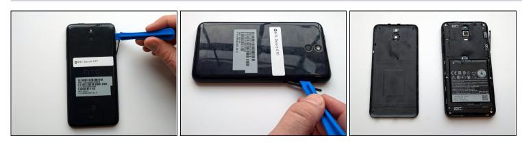
• Using plastic opening tool, take off the back cover of the phone.
