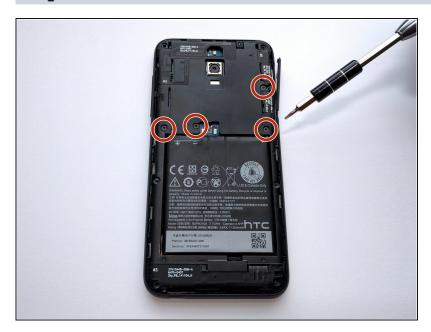
Using Torx T5 Screwdriver, remove the four 4mm black torx screws
