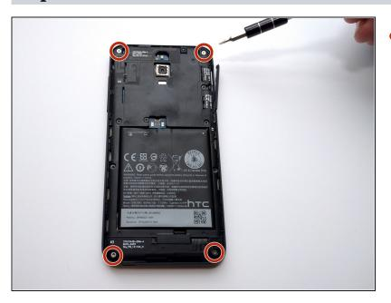
Using Torx T5 Screwdriver, remove the four 5mm silver torx head screws.
