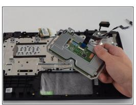
Once unscrewed, use the plastic opening tools to lift and slide out the touchpad. Be careful not to damage the speaker wire that runs across it when removing.
