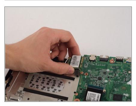
Return to the wireless chip and gently pull it from the connector on the side of the motherboard.
