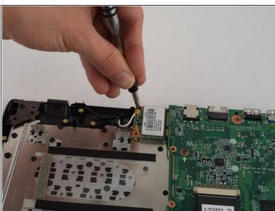
Remove one 6.2 mm Phillips #1 screw from the wireless chip on the left side of the motherboard.
