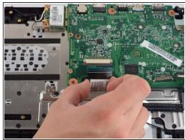
Locate the keyboard cable on the motherboard. Using, two plastic opening tools on each side of the connector, pull the two gray tabs outward and then remove the cable from the motherboard.
