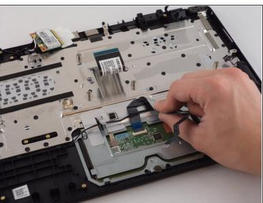
Start by peeling off the touchpad cable that is stuck to the computer.
