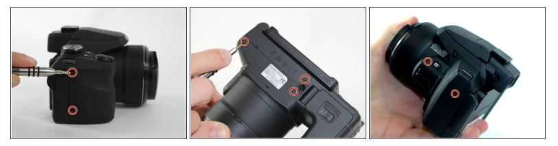
• Remove the 7 screws on the perimeter of the camera body.
