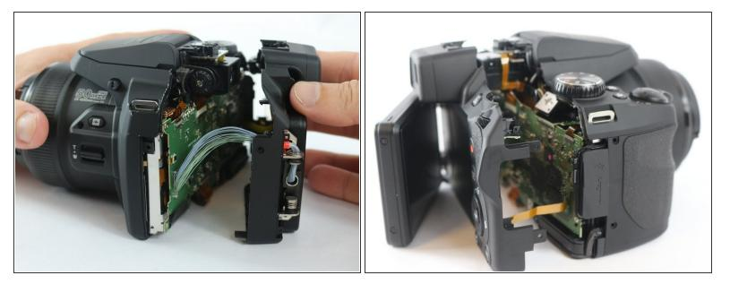
• Carefully pull the back body off of the camera.
