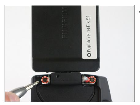
Remove the 2 screws from under the LCD hinge caps.
