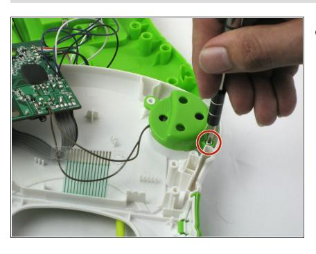
Using a Phillips #00 screwdriver, remove the screw highlighted in the image.
