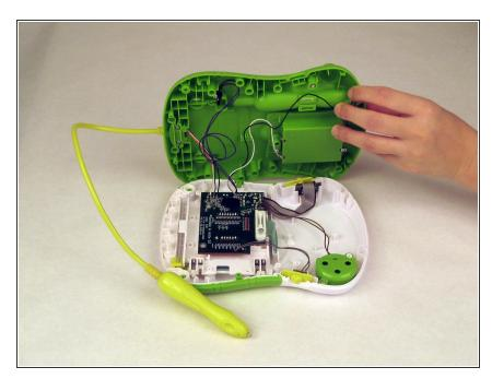
Very carefully, remove the back case to reveal the contents of the toy.
