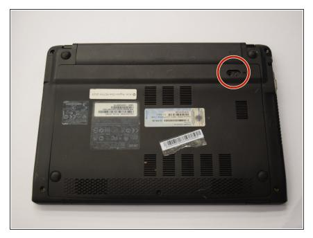
Locate the circular slot positioned at the bottom right of the battery.
