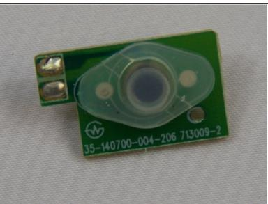
The button/circuit board should be loose now. Gently pull out the button/circuit board to remove it from the device.
