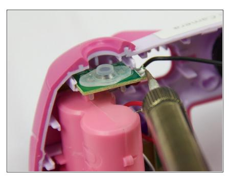
Unsolder wires connected to the right side of the circuit board. Pull the wires to the side.
