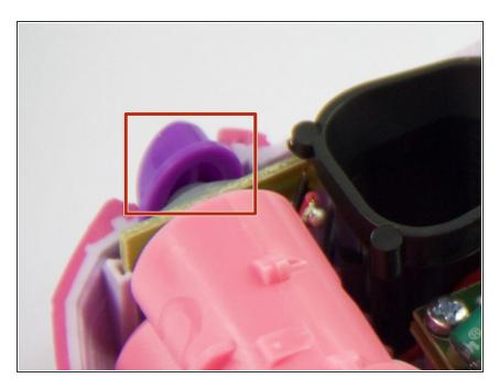
Remove the purple plastic that covers the button and circuit board.
