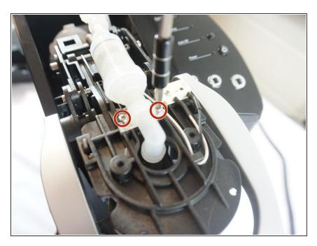
• Unscrew both 1.5mm screws located on the water pump.
