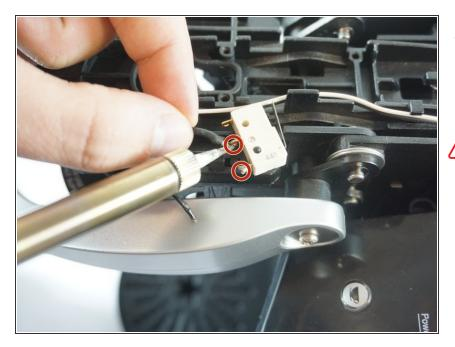
Put the replacement sensor back on the post that holds it and begin to solder the two metal connections back to the sensor.
