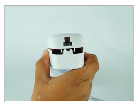
• Pull up on the spudger while simultaneously pulling up the top shell of the phone.
